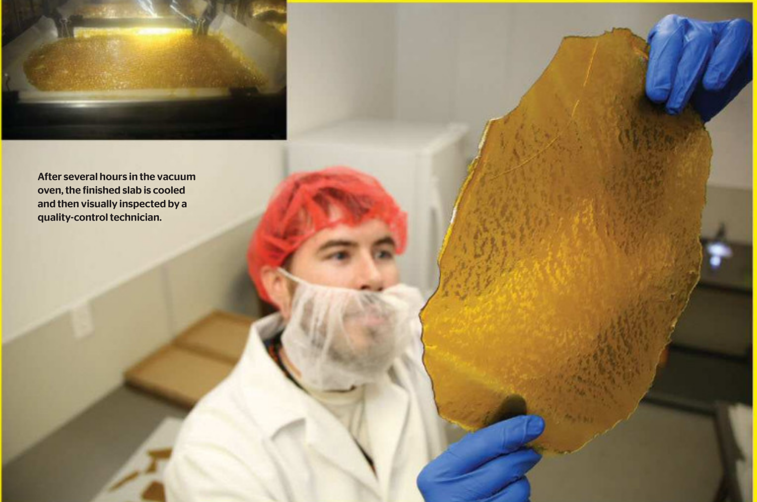
(Above and left) TC Labs uses laboratory vacuum ovens for the next step in the process. The oven introduces heat and pressure to remove the solvent left in the solution. The butane and hash solution will "boil" as the remaining solvent continues to release its bonds.
